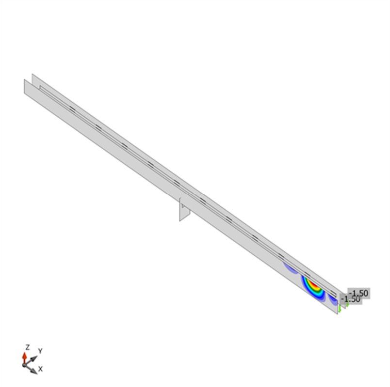
First buckling mode shape, LE1
